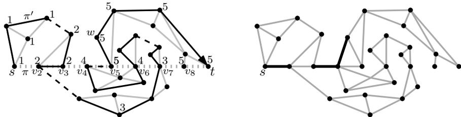
(a) A geometric graph  $G$  (solid gray, solid black and dashed black edges) with an  $s$ - $t$  path  $\pi'$  (black; bridges are dashed). The  $s$ - $t$  path  $\pi$  (dotted gray straight line) belongs to the triangulation  $T$ , which is not shown.
