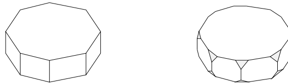
Figure 10: By cutting off the corners of the k -prism, we obtain the polyhedron of N[3, 3, s](k) .
